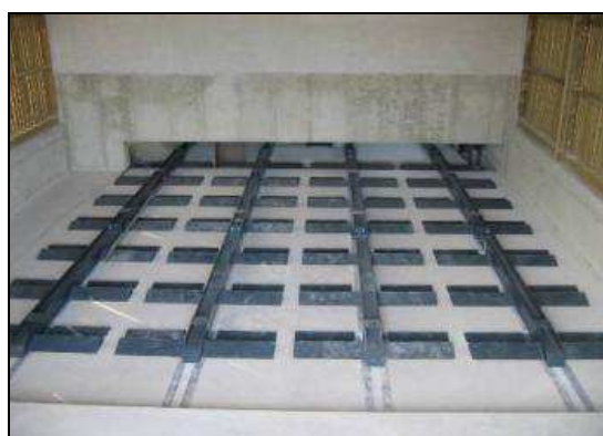
Figure 60. Sliding bar conveyor used for the discharge of silos.
