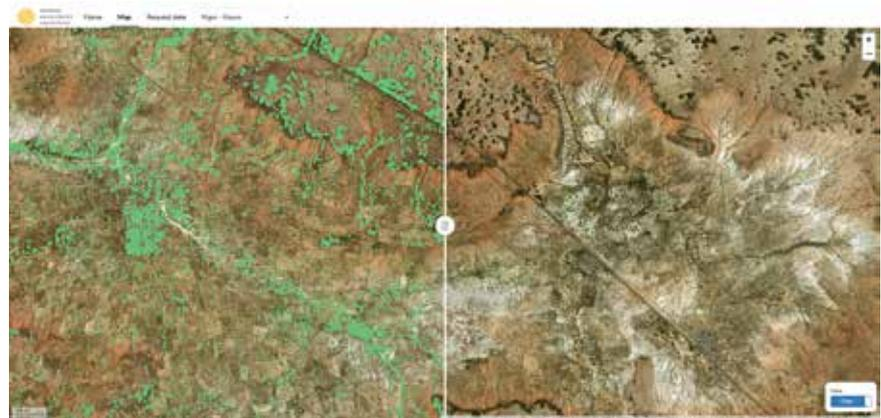
*Note:* A screenshot of the Restoration Mapper prototype, which displays detailed, wall-to-wall maps of the spatial distributions of trees with canopy diameters larger than 2 m. The maps are created using artificial intelligence algorithms and freely available 10-m-resolution satellite data (Sentinel 2). The image on the left shows the pixels of tree cover, and that on the right shows the raw satellite imagery.
