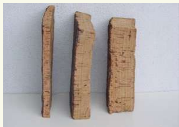
Cork samples with nine years growth showing different thickness and qualities (Credits: UNAC)
