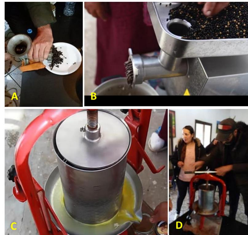
**Figure 11.** Modern extraction equipment: manual chopper (A), electric chopper (B), hydraulic press (C), demonstration (D) (Credits – F. Mezni).
